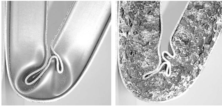
Fig. 17. Cut-through view of empty and filled single-hat beams (left: empty; right: filled).
